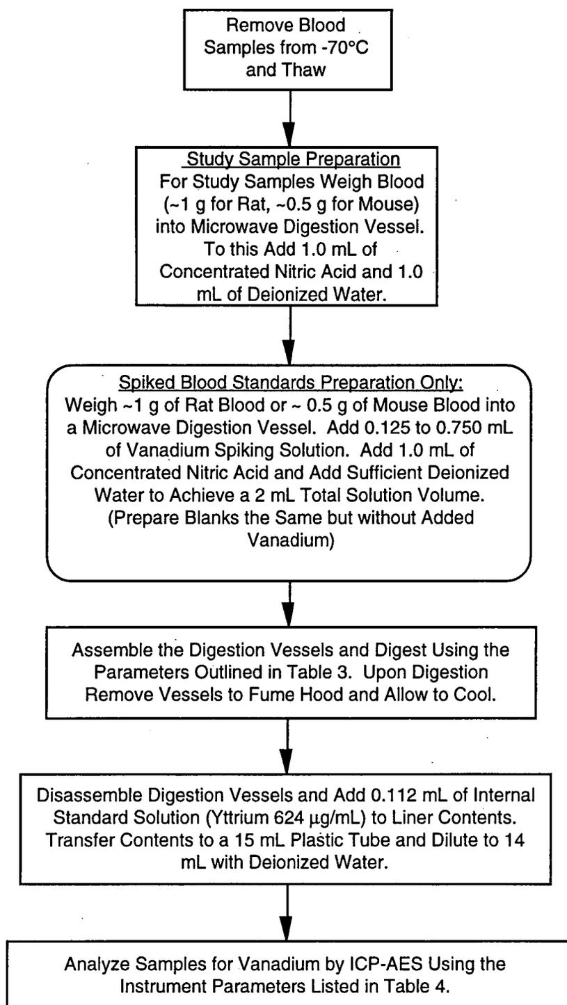
Figure 1. Sample Preparation Scheme for Analysis of Vanadium in Blood
