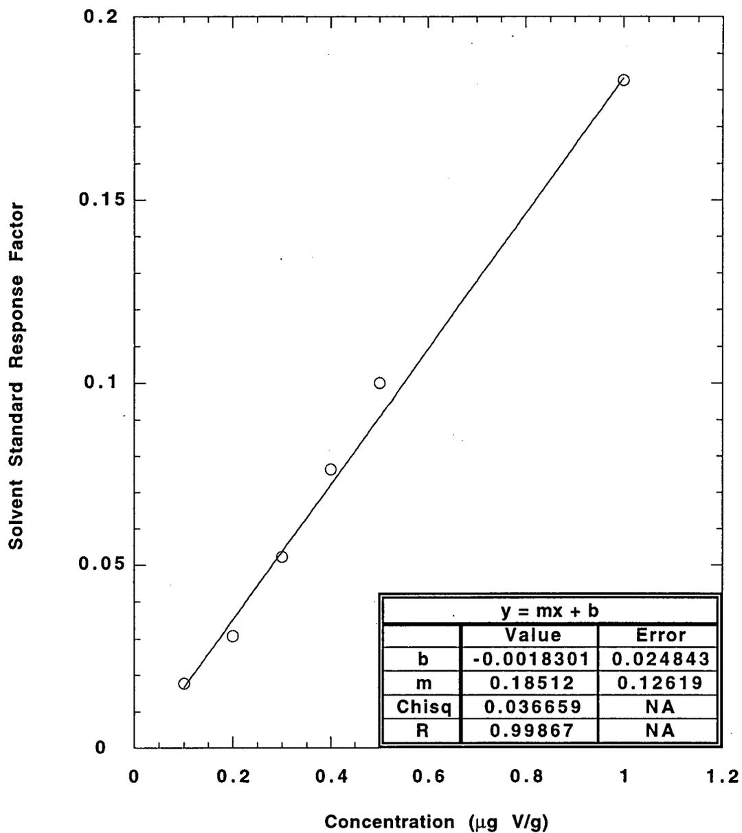
Figure 5. ICP-AES Calibration Curve for Vanadium in Solvent Standards Analyzed with Spiked Mouse Blood Standards
