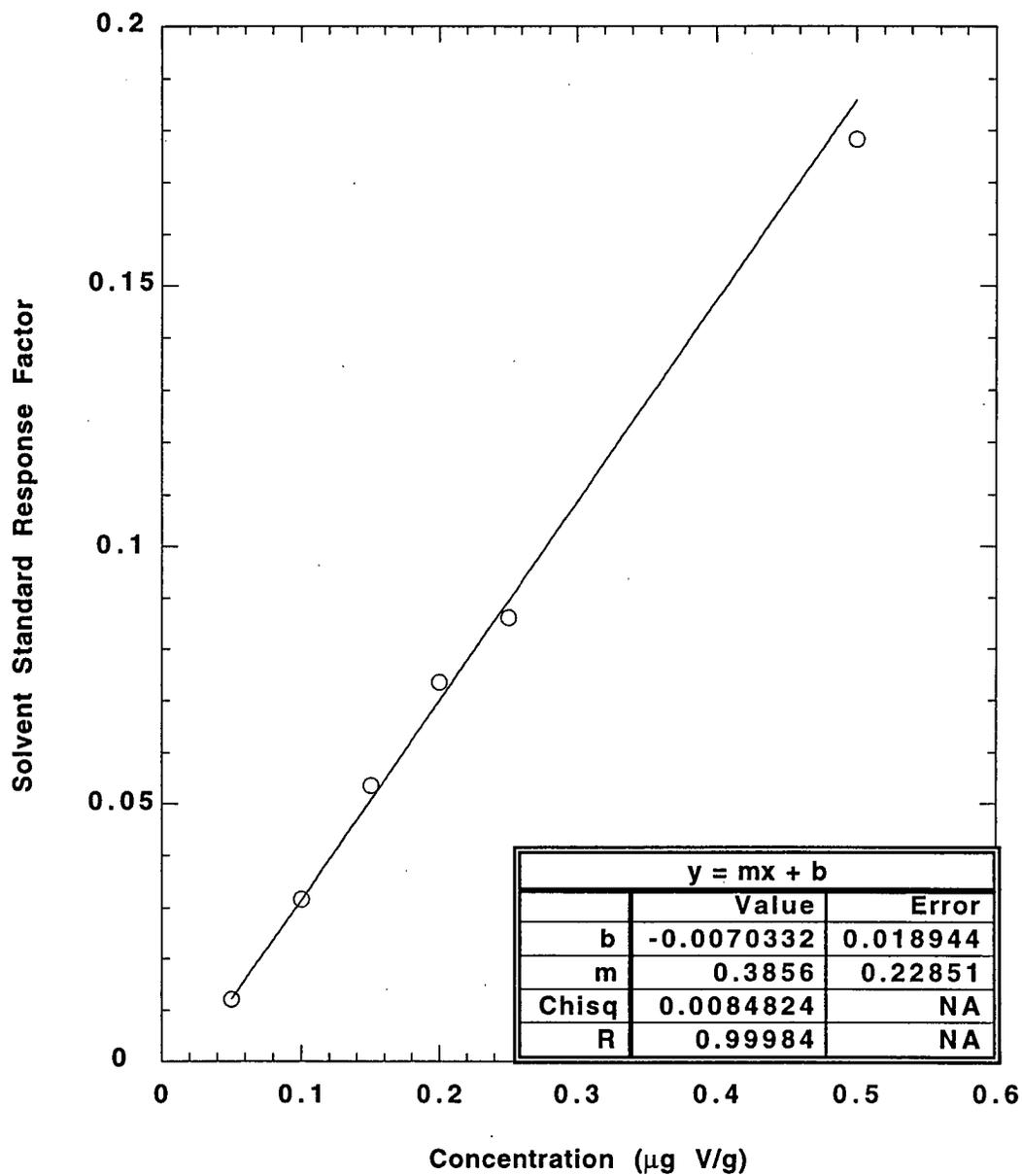
Figure 3. ICP-AES Calibration Curve for Vanadium in Solvent Standards Analyzed with Spiked Rat [Whole-Blood]&A Standards
