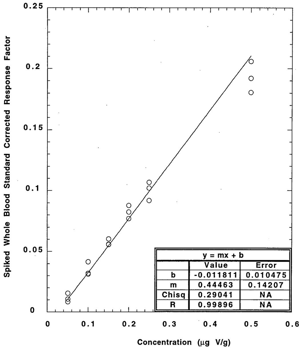
Figure 2. ICP-AES Calibration Curve for Vanadium in Spiked Rat Blood Standards
