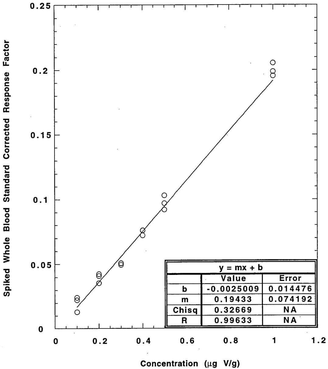
Figure 4. ICP-AES Calibration Curve for Vanadium in Spiked Mouse Blood Standards
