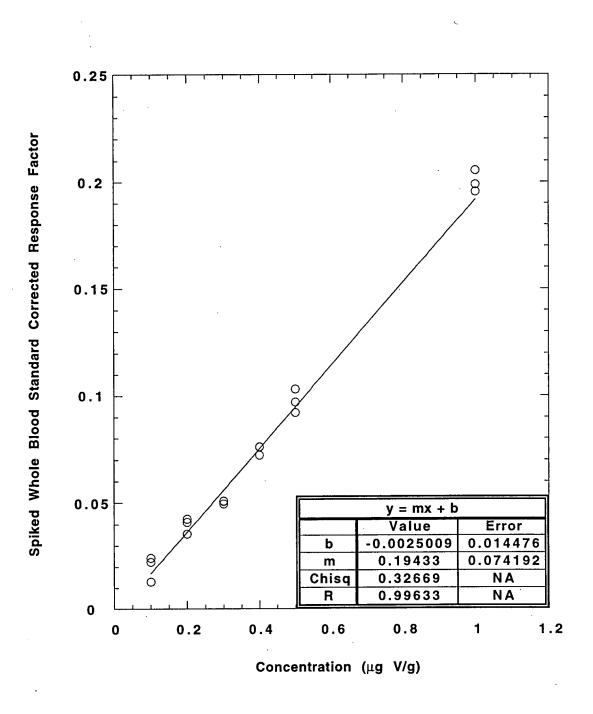
Figure 4. ICP-AES Calibration Curve for Vanadium in Spiked Mouse Blood Standards
