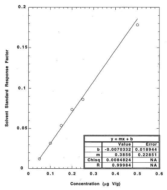
Figure 3. ICP-AES Calibration Curve for Vanadium in Solvent Standards Analyzed with Spiked Rat [Whole Blood]<sup>&A</sup> Standards
