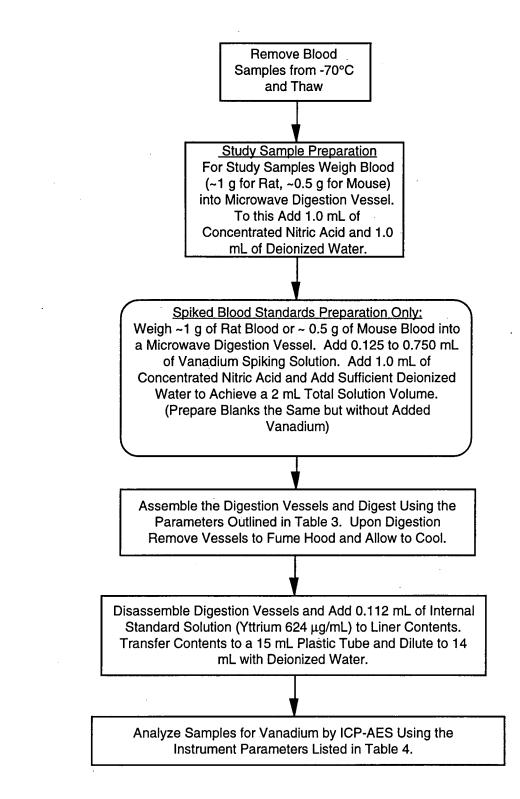
Figure 1. Sample Preparation Scheme for Analysis of Vanadium in Blood
